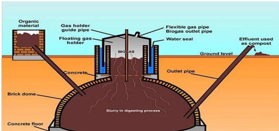
Fig. representing biogas setup
